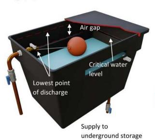
In the case of wholesome water applications, the overflow should be fitted with a screen and light cowl
