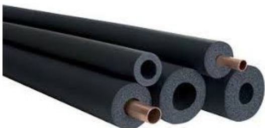
[Expanded Rubber Nitrile Insulation such as Armaflex O - Recommended within a duct at the point of entry. Minimum 19mm wall thickness but thicker required for a shallow point of entry]
